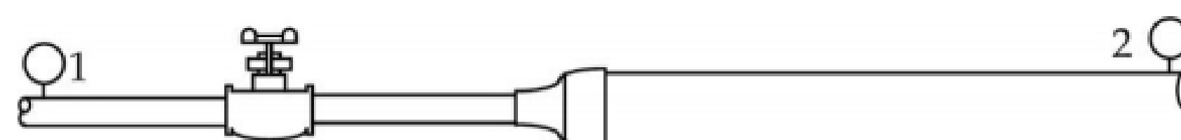
FIGURE 3.11. A series piping system.
